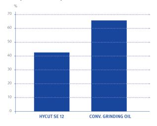
HYCUT SE 12 has a 30 % lower evaporation loss compared to a conventional mineral oil-containing grinding oil of the same viscosity (according to Noak at 150° C).
